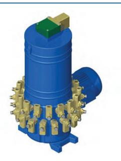
This variable displacement pump is applied for oil and grease lubrication in multiline centralized systems. Displacement of each port can be adjusted separately from minimum to maximum value. It is possible to cut out some of the ports if it is necessary. The number of the ports (from 1 to 30 or 1 to 32 – depending on the variant) should be specified in order. The tank volume in standard execution is 30 dm<sup>3</sup>, but other values . are also available on request.
