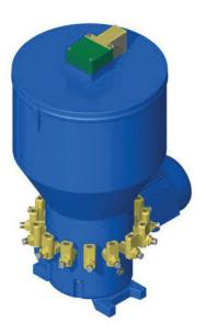
This variable displacement pump is applied for oil and grease lubrication in multiline centralized systems. Displacement of each port can be adjusted separately from minimum to maximum value. It is possible to cut out some of the ports if it is necessary. The number of the ports (from 1 to 15 or 1 to 16 – depending on the variant) should be specified in order. The tank volume in standard execution is 30 dm<sup>3</sup>, but other values . are also available on request.
