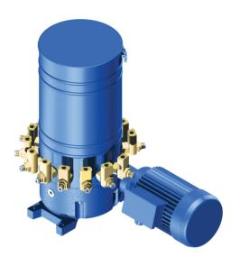
This variable displacement pump is applied for oil and grease lubrication in multiline centralized systems. Displacement of each port can be adjusted separately from minimum to maximum value. It is possible to cut out some of the ports if it is necessary. The number of the ports (from 1 to 15 or 1 to 16 – depending on the variant) should be specified in order. The tank volume in standard execution is 10 dm<sup>3</sup>, but other values . are also available on request.
