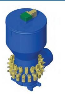
This variable displacement pump is applied for oil and grease lubrication in multiline centralized systems. Displacement of each port can be adjusted separately from minimum to maximum value. It is possible to cut out some of the ports if it is necessary. The number of the ports (from 1 to 30 or 1 to 32 – depending on the variant) should be specified in order. The tank volume in standard execution is 30 dm<sup>3</sup>, but other values . are also available on request.
